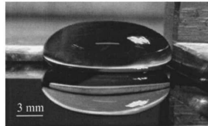
FIG. 2. Large water droplet deposited on a silicon surface at 200^\circ\text{C} .
