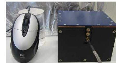
3D imaging of a small volume above it, with a region of interest 15 mm x 15 mm x 10 mm.
